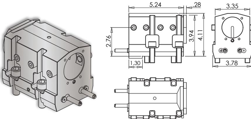
**VELOCITY** ID holders can be used with both internal and external coolant. **Internal Coolant Plates** are included with all **VELOCITY** multitasking turret ID holders.
