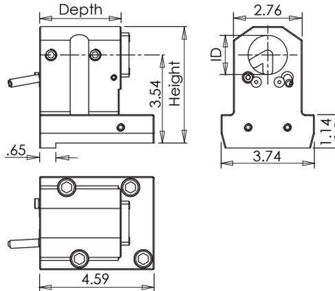
**VELOCITY** ID holders can be used with both internal and external coolant. **Internal Coolant Plates** are included with all **VELOCITY** multitasking turret ID holders.
